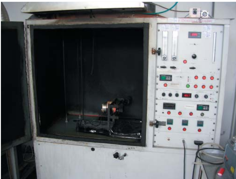
HRR Heat Release Rate - Cone Calorimeter ISO 5660-1
