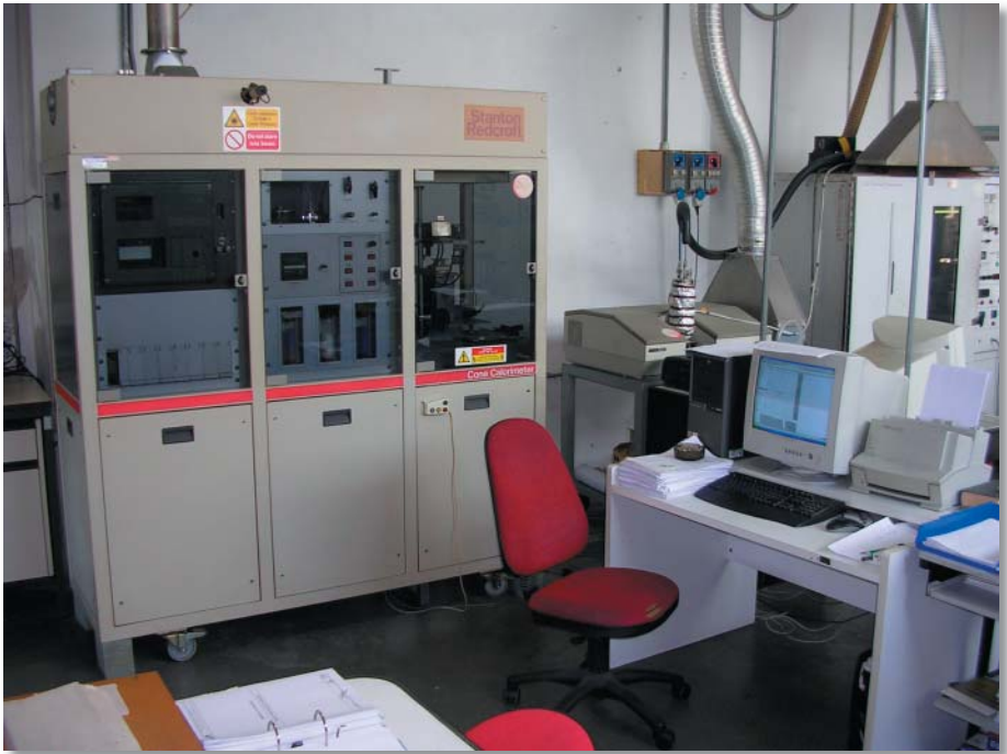
HRR Heat Release Rate - Cone Calorimeter ISO 5660-1
